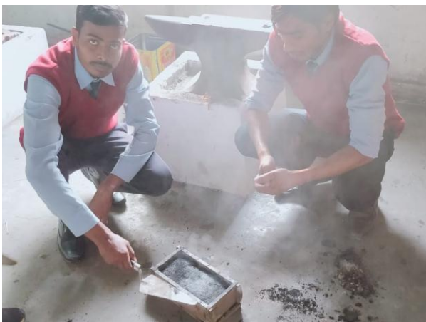
Fig- 6 tamping of brick
