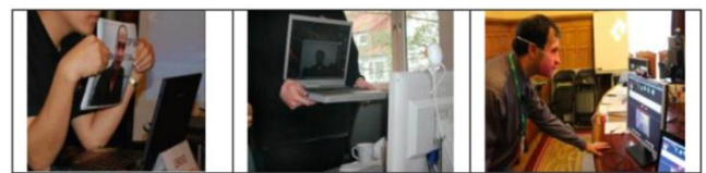
Fig 5: Showing Photo Attack, Video Attack, and Mask Attack from Left to Right respectively.
