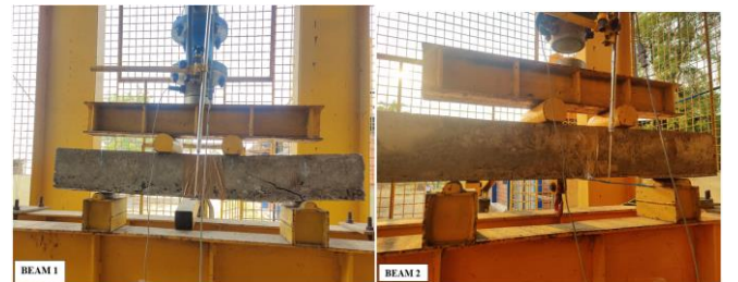
Fig -5: specimens after testing in loading frame
