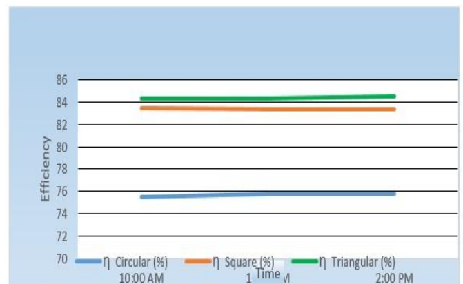
Fig 16: collector efficiency for Circular, Square and Triangular riser tubes
