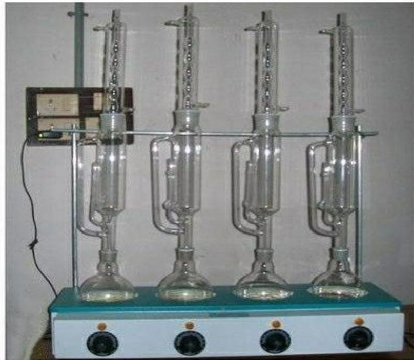
Fig. 1: soxhlet extraction assembly
