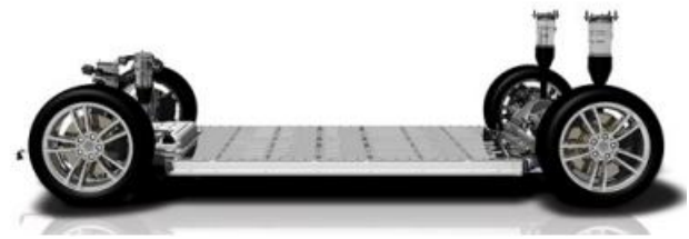
Fig. 8. Battery packing: The battery pack in the Model S is flat and part of the frame that supports the car—the metal case provides structural support
