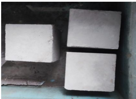
Fig-5 Curing Concrete cubes
