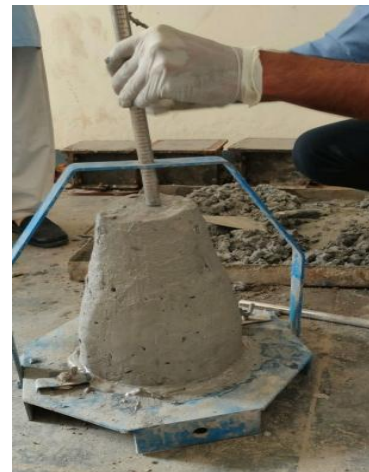
Fig-6 Slump test
