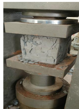
Fig-7 Compression test
