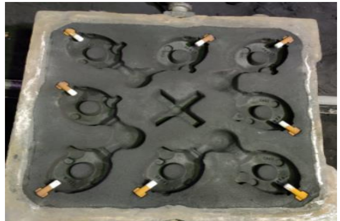
Fig3. Core Arrangement in the cope pattern at the time of molding
