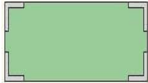
Fig -5: Location of Shear Wall
