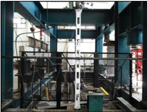
Fig -4: Experimental set-up for built-up batted column
