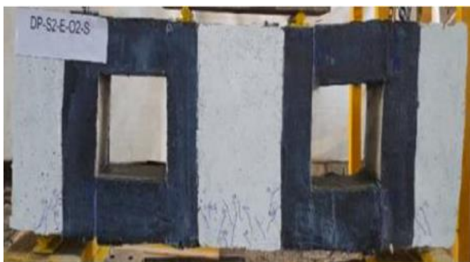
Fig -5: CFRP on deep beam with opening
