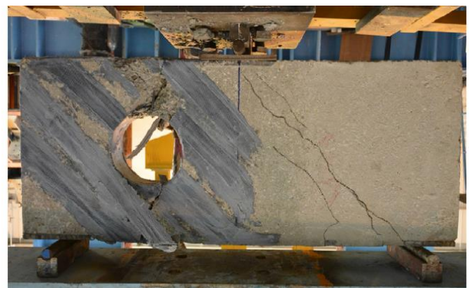
Fig -4: Failure in deep beam with unsymmetrical opening
