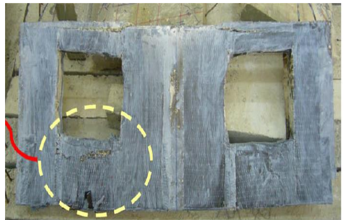
Fig -9: Failure mode of CFRP- strengthened beam
