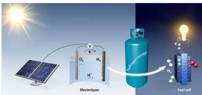
Fig.2. Hydrogen generation using solar via Electrolysis
