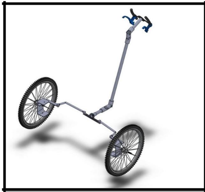
Fig: fully assembled steering(designed on SOLIDWORKS)
