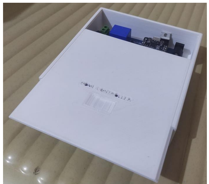
Fig -10: 3D printed sliding case
