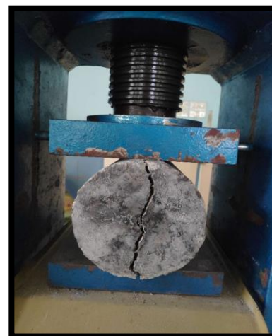
Fig. 7: Testing of Specimen for Split Tensile Strength
