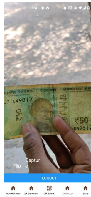
Fig -3: The currency detector helps the visually impaired people to recognise various indian currency notes and gives the voice output for the user.
