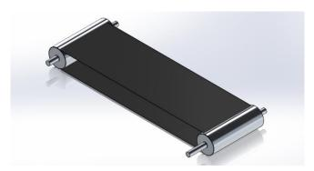
The conveyer belt is used for the unloading of the manufactured pencils. A Flat Belt Conveyor is used for pencils which are rolled after it is glued is taken through the storage for finishing purposes after drying of pencils. This belt is passed through the pressure plate and surface plate for the rolling of pencils and an end drive is used for this conveyor.
