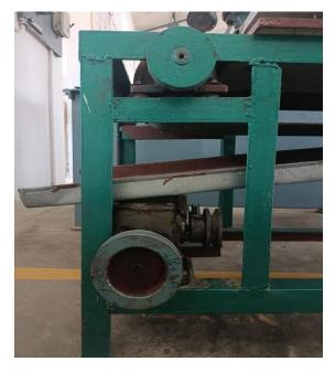
Therefore input shaft speed (N1) = 1500 rpm and the teeth in worm spur gear (Z1) = 37.
