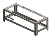
An L-shaped angle rod is used for the construction of the frame. 2.5 - 3 mm thickness is used in concern of load factor. The machinery we are about to manufacture is a light-duty machine.
