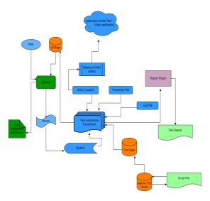
The heart of the system is the Test Automation framework. It's a java-based structure and selenium is used for UI automation. TestNG is the framework used for testing and reporting purpose.
