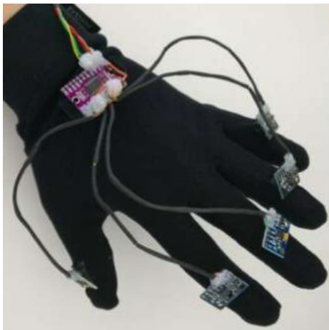
Figure 3: Gloves with flex sensor mounted on it
