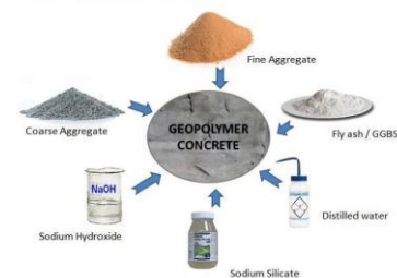
Fig. 3.2 Constituents in Mix design of Geopolymer Concrete
