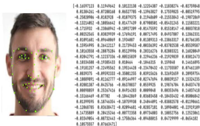
Fig. 9. 128-valued face encoding vector array
