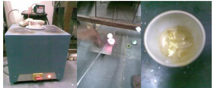
Fig-1: The preparation of ZnO-Na 2 O-Bi 2 O 3 -B 2 O 3 glass system.
