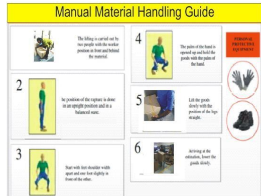
Fig 6.3.3- Modification of manual material handling
