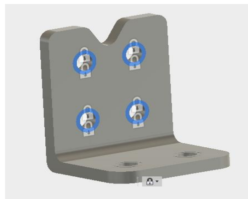
Fig. 2.7: Boundary conditions for modal analysis for iteration 4
