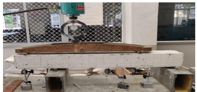
Figure -6: Crack development in Beam with curtailed reinforcement
