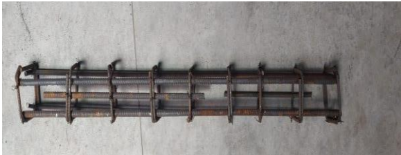
Figure -2: Reinforcement with curtailment
