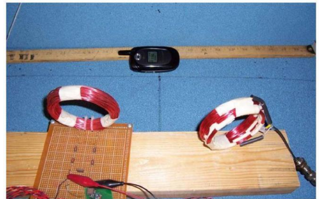
Fig 4. Magnetic coupling test set-up
