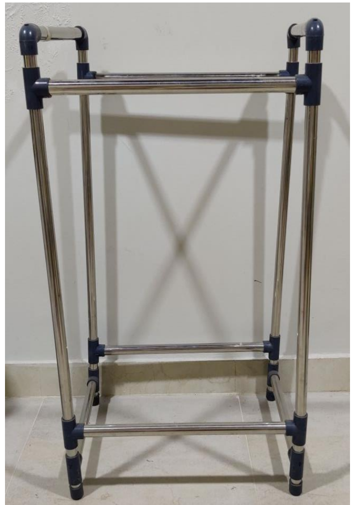
Fig. 6 Stand of the Multipurpose Sanitization Chamber
