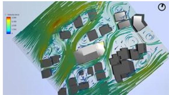
Figure 32 Wind flow analysis – Plan (Source: Author generated)
