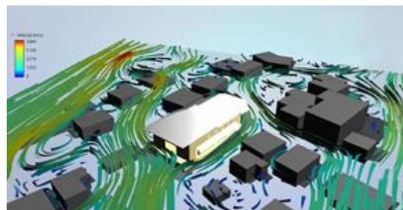
Figure 33 Wind flow analysis around the South façade (Source: Author generated)
