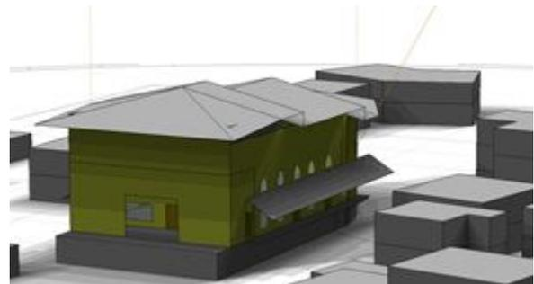
Figure 28 Shadow range on South Facade for April (Source: Author generated)
