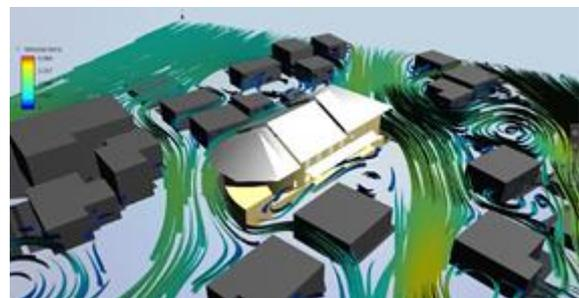
Figure 34 Wind flow analysis around the North façade (Source: Author generated)
