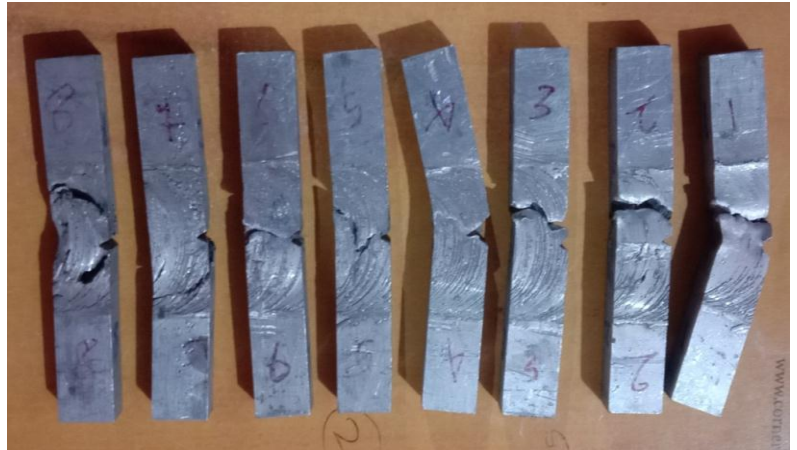
Figure 3.3: Impact test specimen after break
