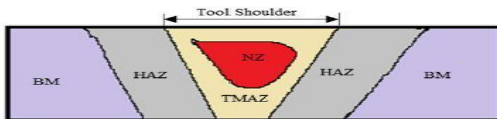
Figure 3.4: Figure showing the different zones of FSW.
