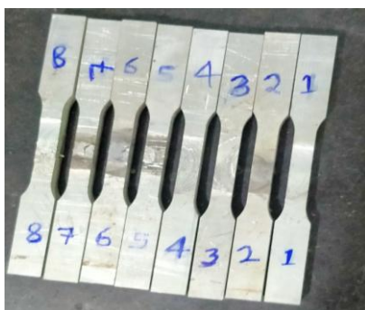
Figure 2.7: samples for tensile test after EDM wire cut machine
