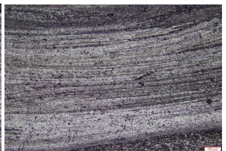
HAZ Weld at 200X
