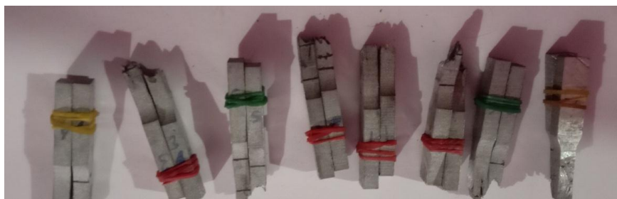
Figure 3.2: Tensile Test specimen after Break.
