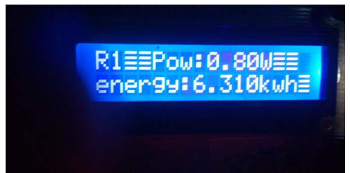
Fig -11: Results being displayed on LCD for Room 1
