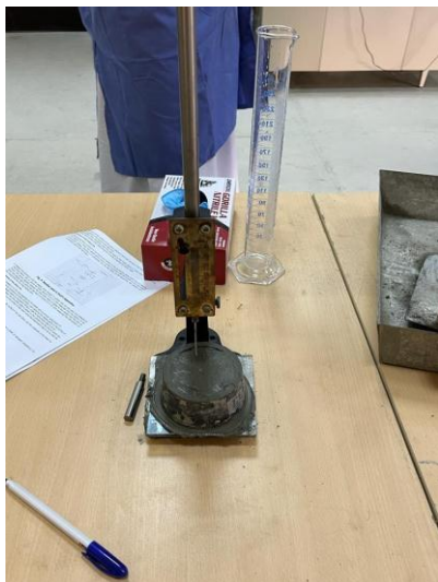
Figure -4: Setting time test on cement
