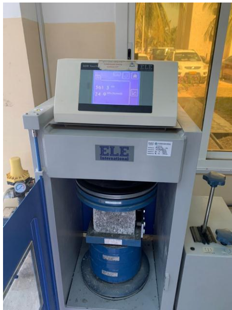
Figure -5: Compressive strength test
