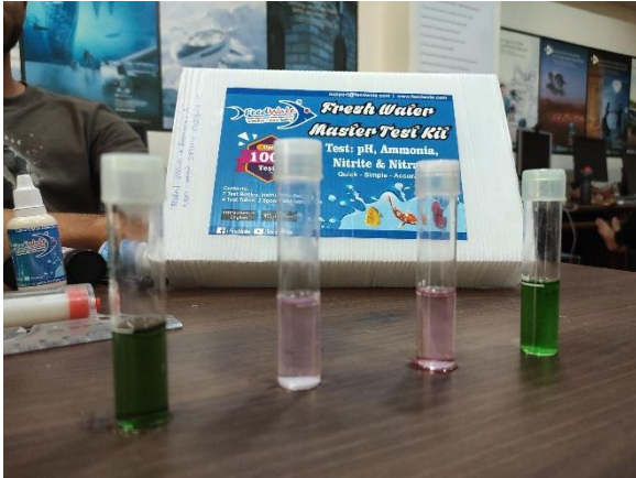
Fig 26: Day 05 – readings showing ammonia spikes in culture tank with maintained PH level
