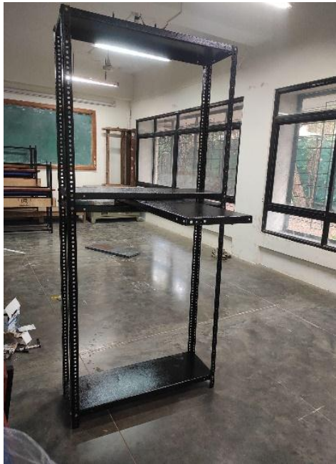
Fig 16: Assembled Rack for biological and mechanical filter setup
