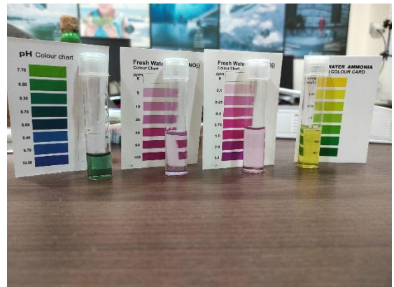
Fig 27: Day 28 – Result showing stable levels for ammonia, nitrite, nitrate, and PH
