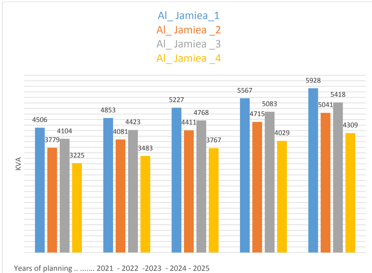
Fig. 7.2 Al_Jamiea network (Load growing feeders)
