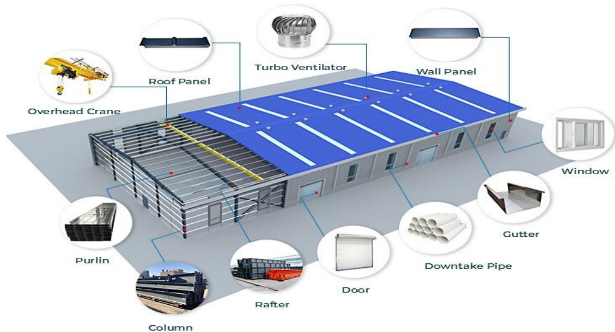
Figure 1 Pre-Engineered steel Structure
