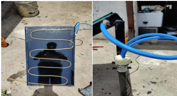
Figure 42 Experimental Modal Solar flat plate collector single copper tube with steel collector & Figure Water motor
