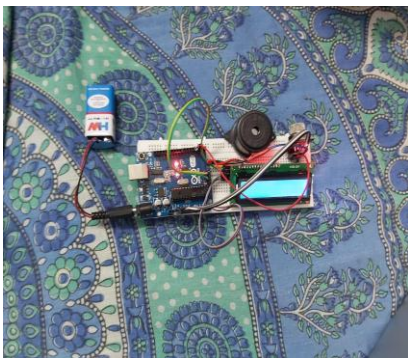
Figure.9 Prototype model of the gas leakage detection system
