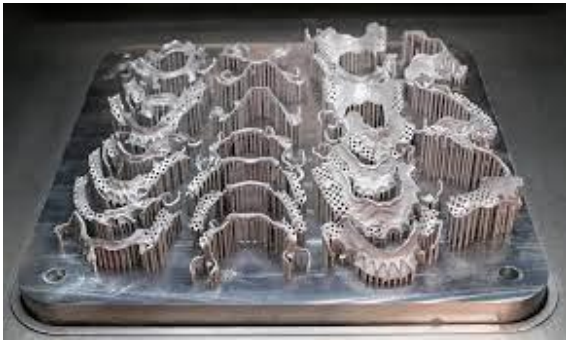
Figure 7: Dental parts printed in metal 3D Printer.
