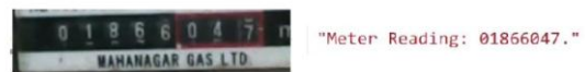
Fig -13: Image Processing using Node-Red with Raspberry Pi incorporating Google Vision API
