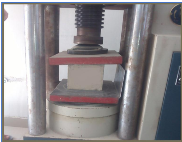
Fig. 2: Compression testing machine (CTM) used for study
