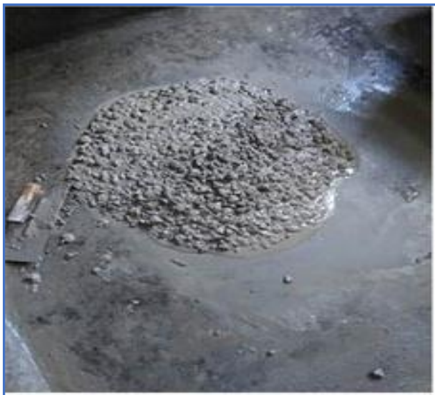
Fig. 1: Slump Flow Test
