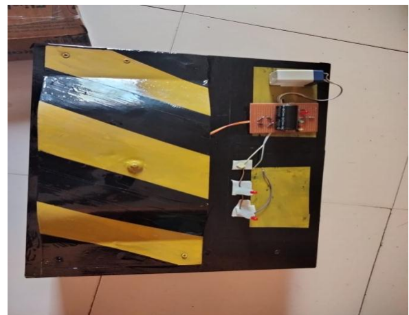
Fig 2:prototype model picture of road power generation using method of speed breaker
