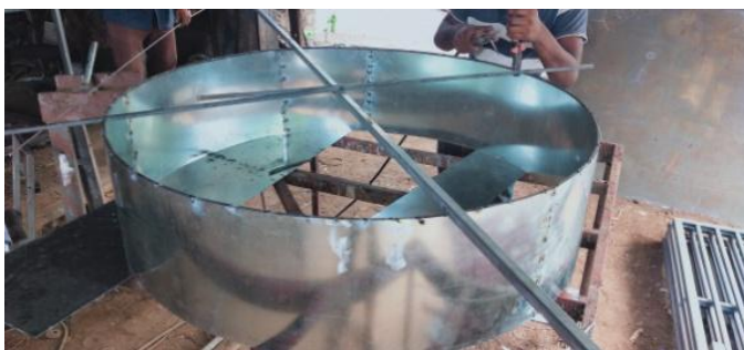
Fig -2: Fabrication of propeller casing
