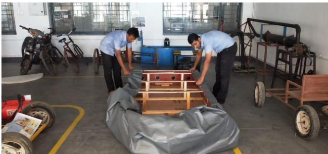
Fig -3: Assembling the hovercraft skirt
