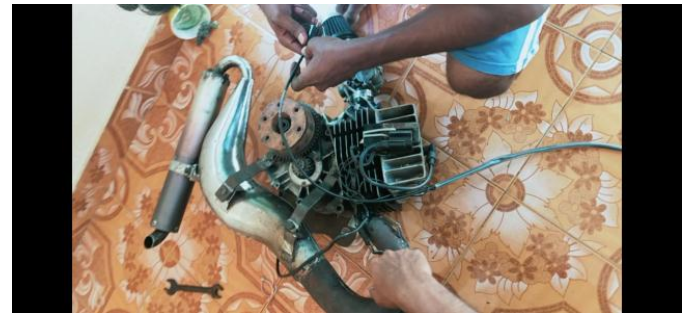
Fig -4: Modified Shogun engine for the hovercraft
