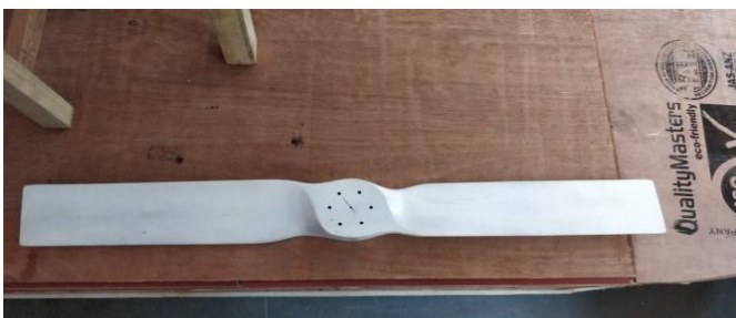
Fig -1: Finished wooden low-pitch two-bladed propeller
