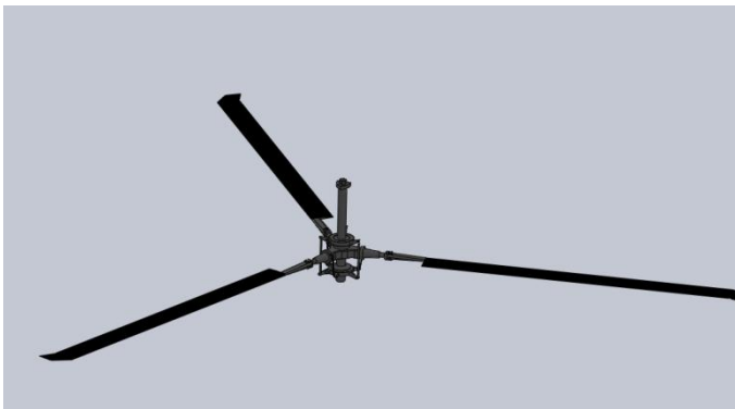
Figure 8 : 3D MODEL Assembly of Helicopter Main Rotor Head
