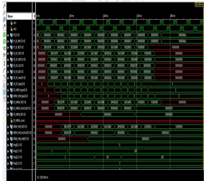
Fig.8 Simulation result for the program to verify register manipulation
