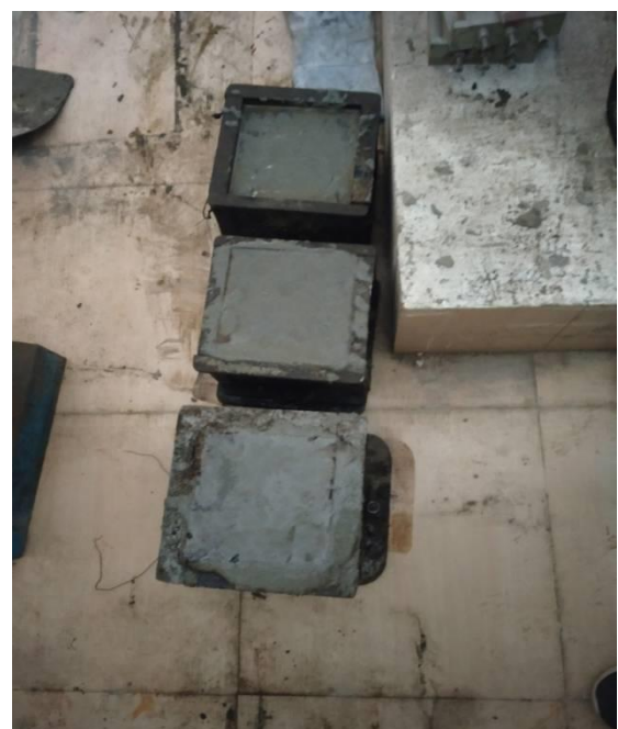
Figure-2: Casting of cube specimence
