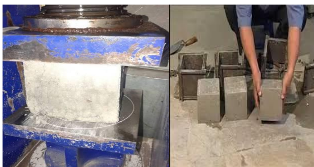
Fig 3.1 Cubes testing for compressive strength
