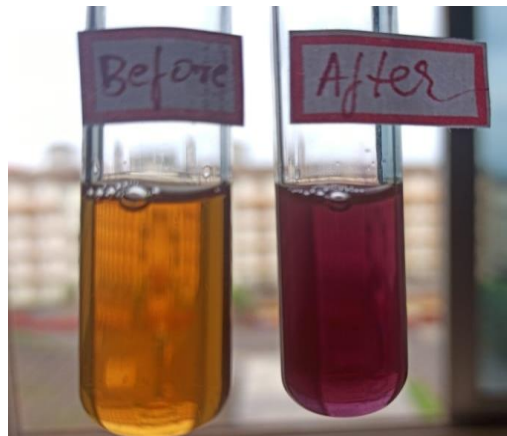
Plate 01: Color changed after adding auric chloride
