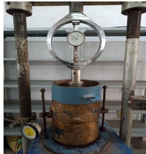
Figure-2: CBR test apparatus
