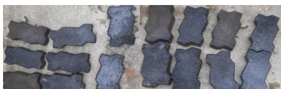
Fig-6: Paver block under acid test
