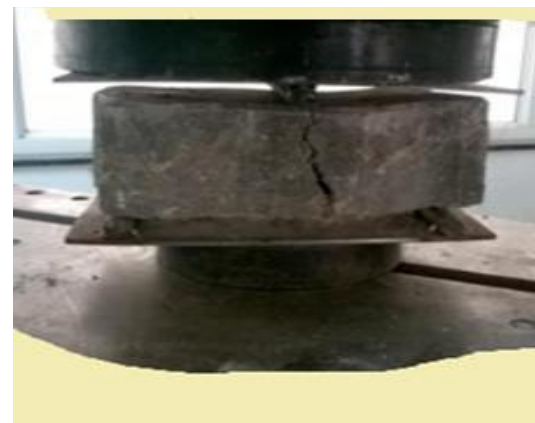
Fig-5: Paver block under flexural loading
