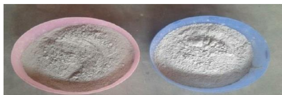
Fig-2: Fly ash and glass powder after being sieved to 300 µm and 90 µm
