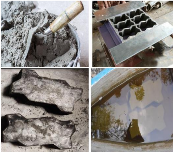
Fig -3: Procedure for making the paving block (a) mixing; (b) molding; (c) demolding ; (d) curing method.
