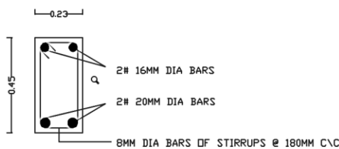
Fig -6: Reinforcement details of Beam
