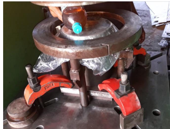
Fig -6: Applying oil on punch
